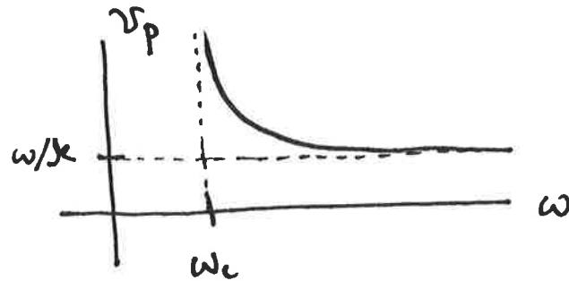
The phase velocity is  $\omega/k$  for large  $\omega$ ,
